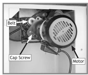
Figure 86. Motor mount cap screw.
